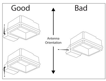
Figure 1 - Proper Antenna Installation
