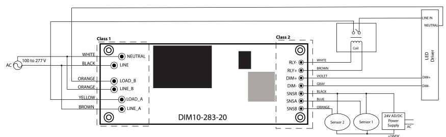
Figure 2 - 100 - 277VAC Wiring Diagram
