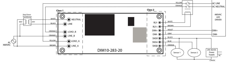
Figure 3 - 480VAC Wiring Diagram
