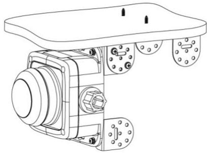
The drawings below demonstrate how to assemble the bracket so that the sensor is positioned at 90° relative to the mounting surface.
