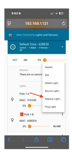
Step 5 – Enter the new SNAP address. In this example, 65bd04 is the MAC address of the replacement controller. Enter this value and then select the REPLACE button. The MAC address can be found on the sticker pack included with the new controller.
